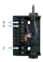
First remove the old cable connection. Once you have disconnected the old cable connection, reconnect the cables as described in chapter 4. Loosen the two screws used to fasten the old mounting flange. The screws must be kept for further assembly. The previous flame monitoring device can now be removed. Then remove the old mounting flange. The KLC mounting flange can be replaced directly and fastened with the old screws.
